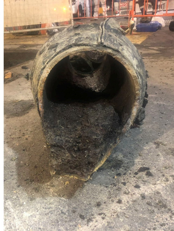
Old Cast Iron Main Clogged with Debris
