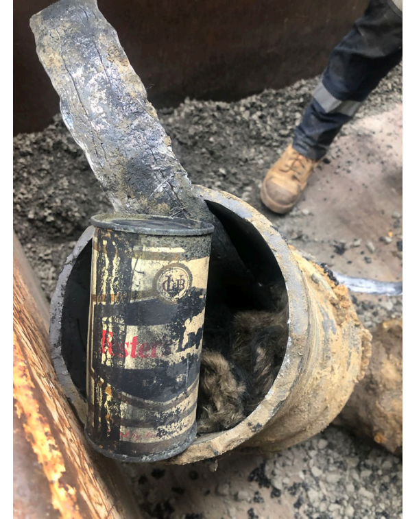
Elbow Blockage that was Cut-out Lt Collins St SE1 - Comdain
