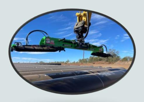
Spreader bar arrangement above. Vacuum chamber is located within the spreader bar and hangs off the rotator and hitch. This set up reduces the SWL by the weight of the spreader bar and shoes.
