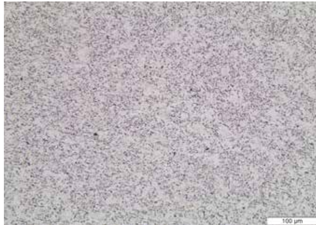
API 5L X52. Fine-grained ferrite with a fine pearlite carbide structure
