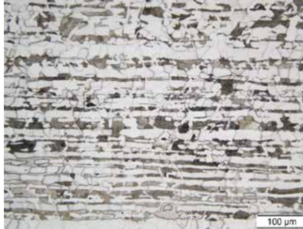
API 5L X42. Pearlite and ferrite in a heavily banded structure
